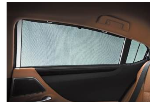
clear field of view when reversing, the rear window sunshade automatically lowers when reverse gear is engaged.
